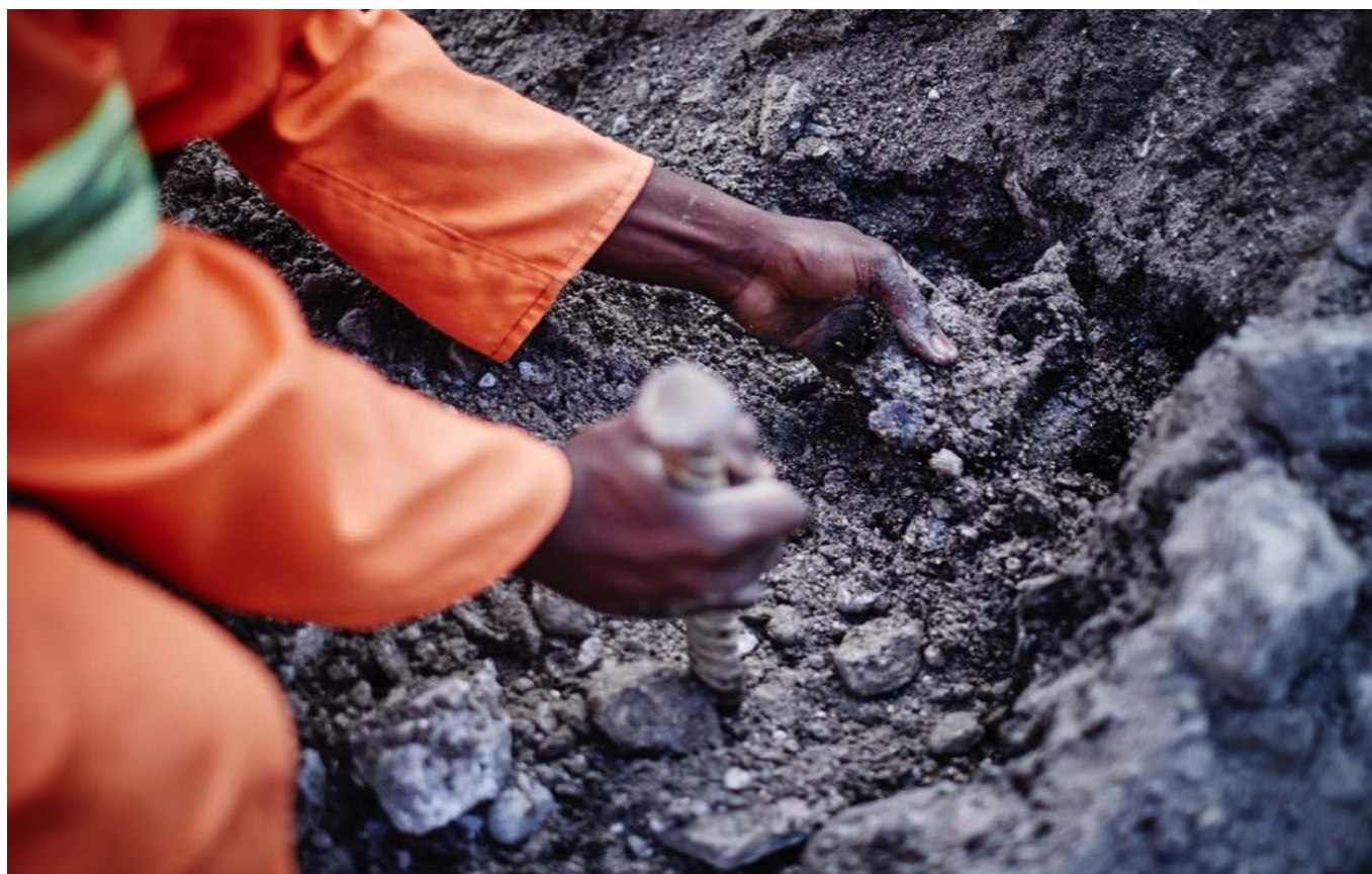
Not all primary bedrock deposits are hard. Here emeralds are hosted in soft talc magnetite schist, a type of metamorphic rock, where they can be sifted out by hand, preserving the integrity of the gemstone. (Photo courtesy of Gemfields.)
