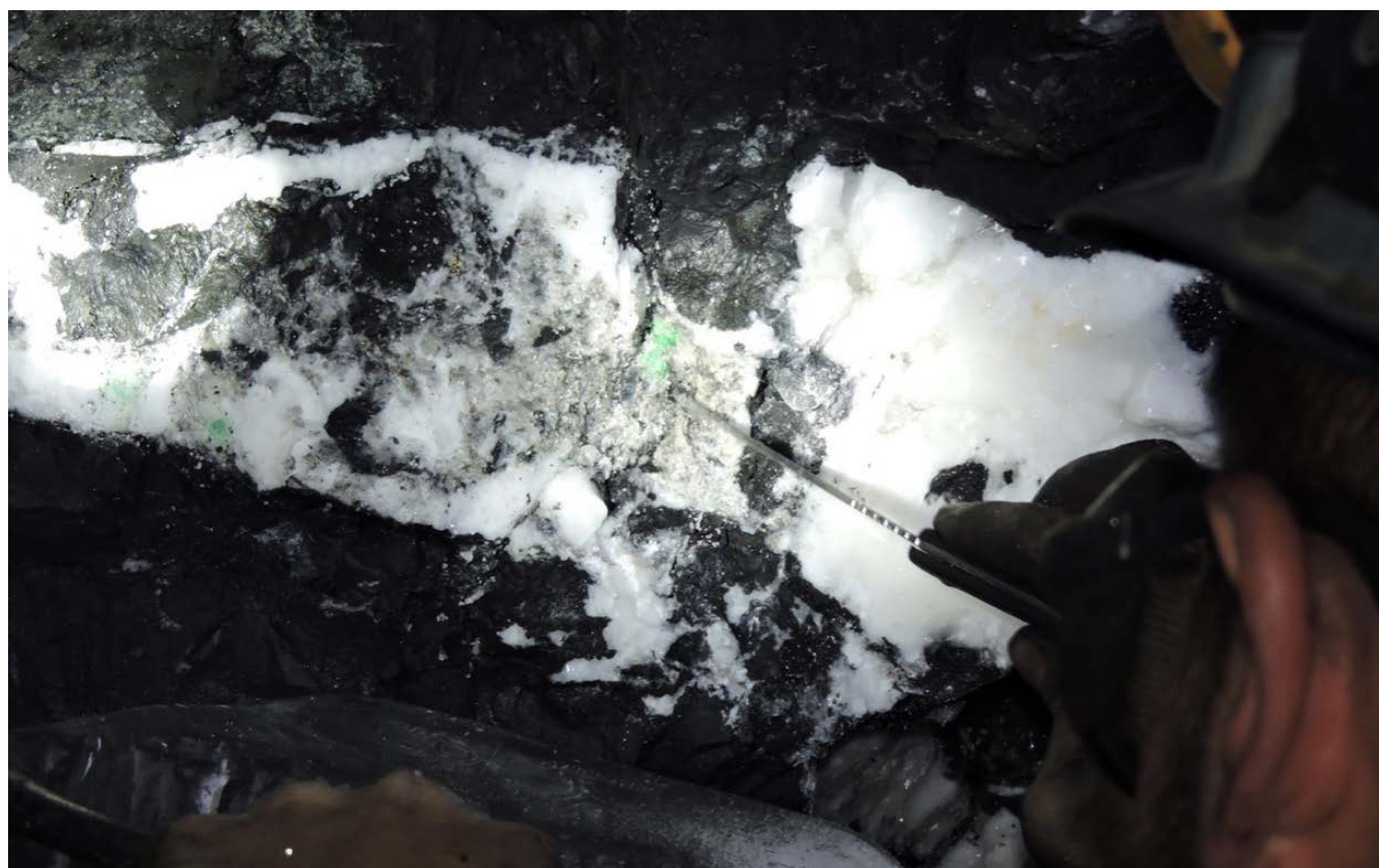
An emerald being removed from a large-scale underground mine in Colombia. This is an example of a primary deposit where emeralds are hosted within veins. (Photo courtesy of Muzo Emerald Colombia).
