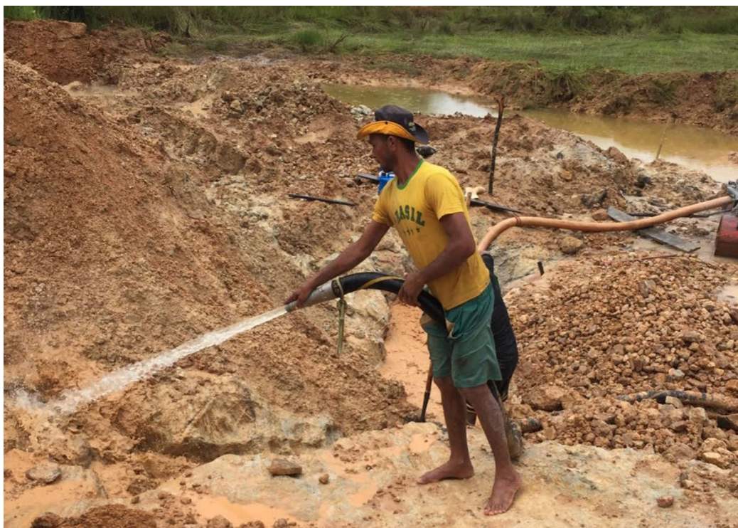
Hydraulic mining at a secondary, alluvial gemstone deposit. High pressure water jets are used to free up loose material and release gemstones. (Photo courtesy of Swarovski.)
