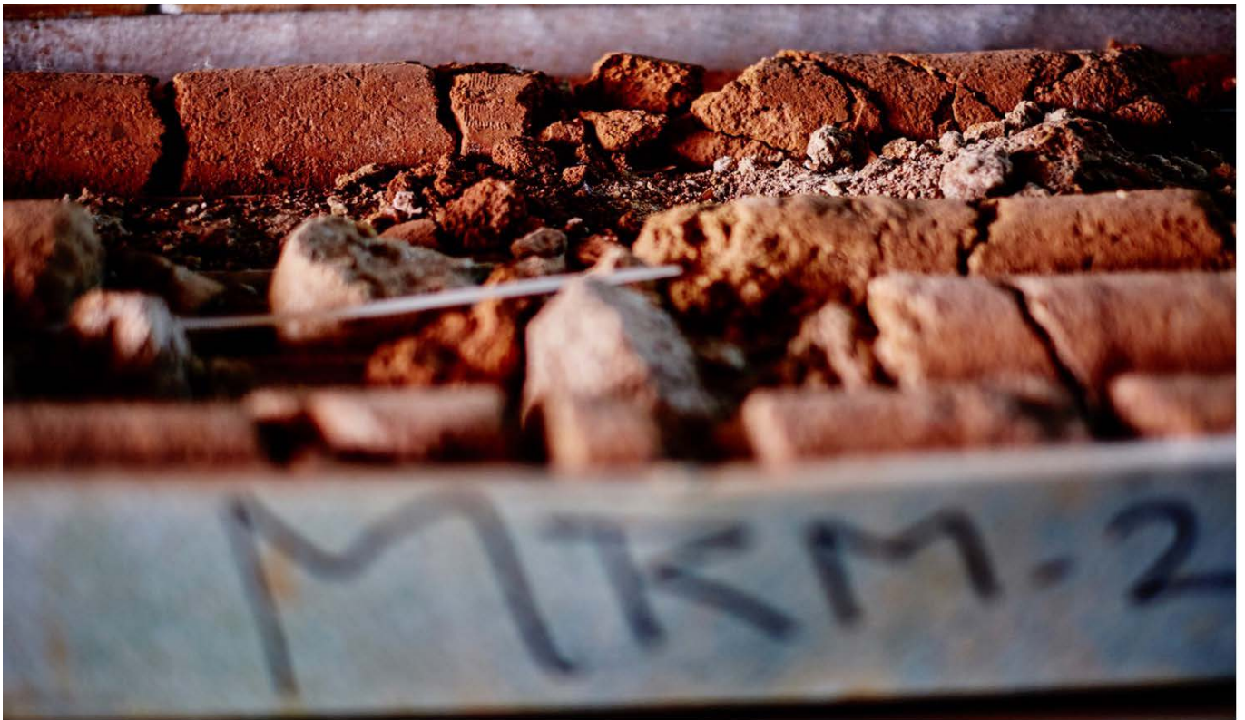
A drill core sample from exploration at the Montepuez ruby mine, Mozambique. Drilling is an example of an advanced exploration technique used to reveal information from below the surface. (Photo courtesy of Gemfields.)
