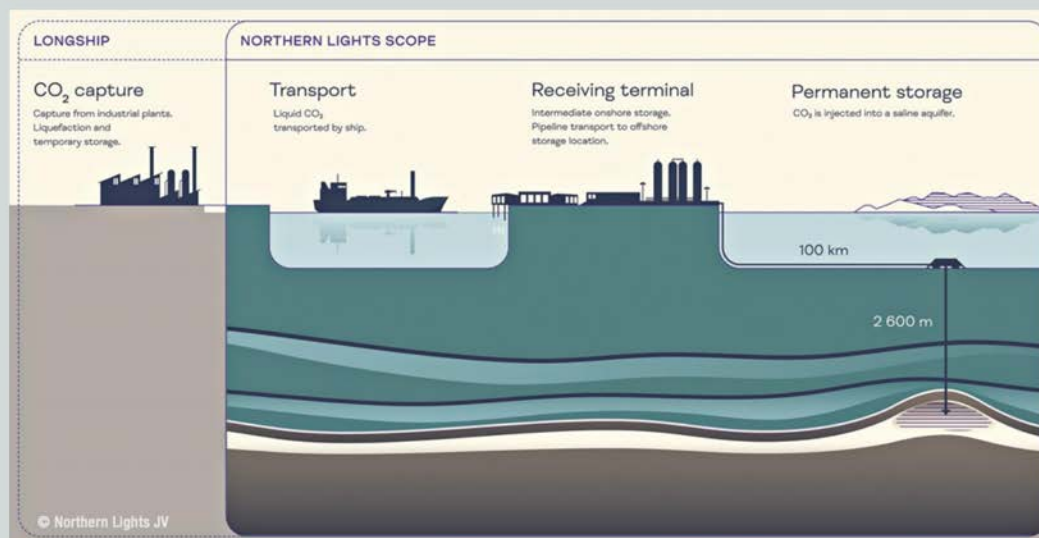
Figure 15: The Longship CCS value chain of the Northern Lights Project
